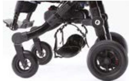
935 Oxygen bottle holder. Only for outdoor base.
