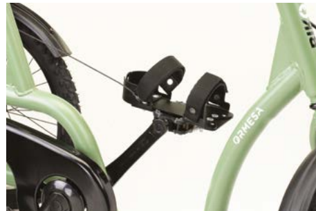
841 Pedal cage with length and width adjustable foot imprints and fastening straps, with support kit. It can be ordered per piece.
