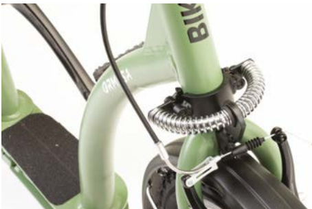
882 Steering limiter with spring.
