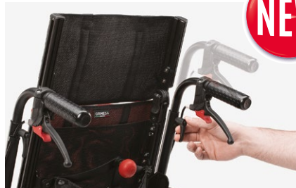
951 Height adjustable push handles. TOOLS FREE! It increases the total height of max. 7 cm/2,7 in (94-101 cm/37-39,7 in).
