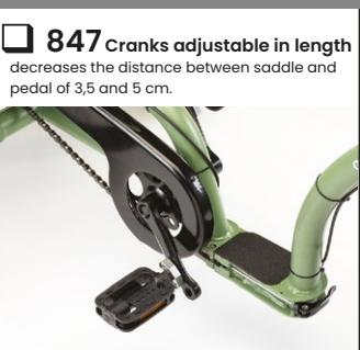
847 Cranks adjustable in length decreases the distance between saddle and pedal of 3,5 and 5 cm.
