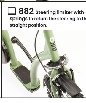
**882** Steering limiter with springs to return the steering to the straight position.
