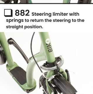
882 Steering limiter with springs to return the steering to the straight position.
