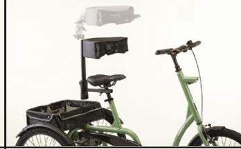
842T Trunk support, adjustable in height, inclination and backward-forward with belt and joint.
