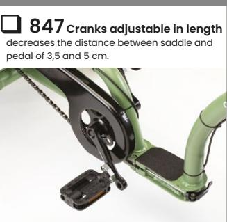
847 Cranks adjustable in length decreases the distance between saddle and pedal of 3,5 and 5 cm.
