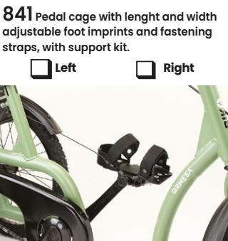
841 Pedal cage with length and width adjustable foot imprints and fastening straps, with support kit.
