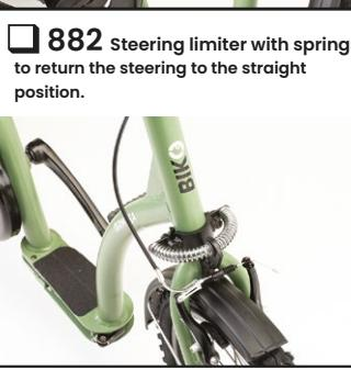
882 Steering limiter with springs to return the steering to the straight position.
