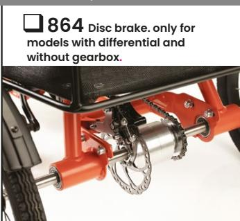
864 Disc brake. only for models with differential and without gearbox.
