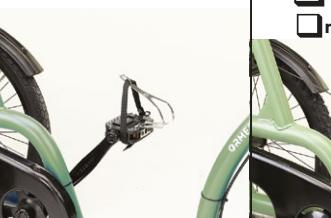
841 Pedal cage with length and width adjustable foot imprints and fastening straps, with support kit.
