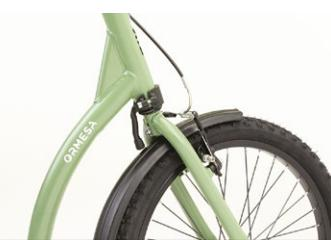
882 Steering limiter with springs to return the steering to the straight position.
