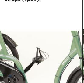
841 Pedal cage with length and width adjustable foot imprints and fastening straps, with support kit.
