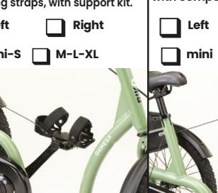
846 Ankle support adjustable in height, with support kit. Only with component 841.
