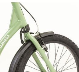
882 Steering limiter with springs to return the steering to the straight position.
