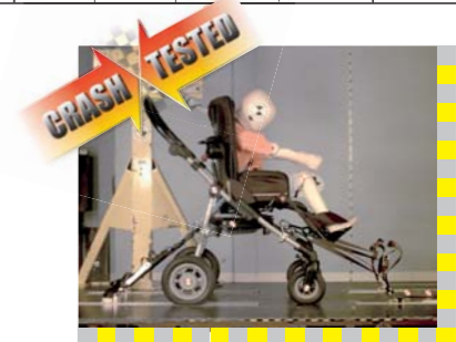
BUG with base 869 passed CRASH TEST according to the ISO 7176-19 and ANSI RESNA WC/19
